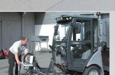
Quickly ready for use: Thanks to the quick-coupling triangle allowing easy and back-friendly changing of attachments without
